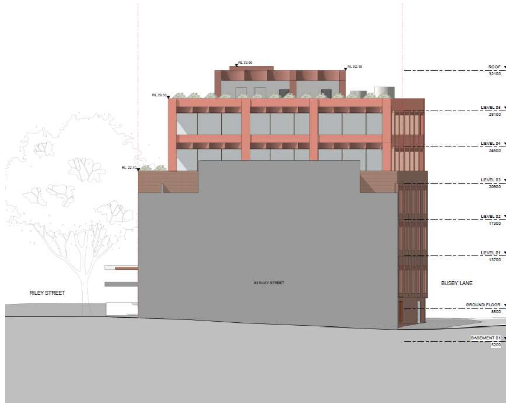
Figure 50 - Northern elevation of a building form supported by the proposed building envelope. (Source: SJB)
